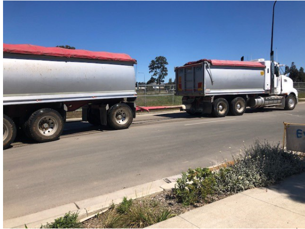
Photos 3 & 4: Covered load of spoil and drain controls on Conferta Avenue
